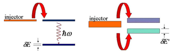
FIG. 1. (Color online) Cartoon of population injection in mid-infrared (left) vs terahertz (right) structures. Population inversion can be easily achieved on the left but not on the right. In this case, the electrons can tunnel to either the upper or lower levels: it is difficult to achieve population inversion in terahertz intersubband-based devices.
